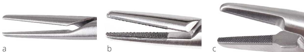
Fig 2-14 (a to c) It is advisable to use needle holders with non-serrated jaws when using thin suture threads to avoid damage to the thread structure (a). Serrated jaws may damage the structure of 3-0 or thicker threads, but would not cause them to break (b). Tungsten-carbide coating of the jaws and joint prevents corrosion on the beak of the needle holder caused by prolonged usage (c).
